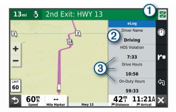
Diagnostic and malfunction indicator. Select to view detailed information about diagnostic or malfunction alerts (*Viewing Diagnostics and Malfunctions*, page 46).
