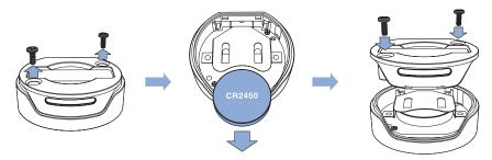
STEP1. Unscrew the back panel of the SOS Button
