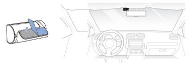
(E) Adjust the angle of the lens by rotating the body of the fror We recommend pointing the lens slightly downwards (≈ 10° below horizontal), so as to record video with a 6:4 road to background ratio. Tighten the screw fully.
