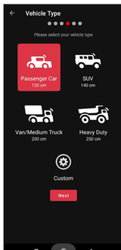
19. To set the "camera height" (from ground), select the picture that is most similar to the vehicle type you are installing KP2 onto. If you prefer to enter a more precise measurement, please choose the Custom option.
