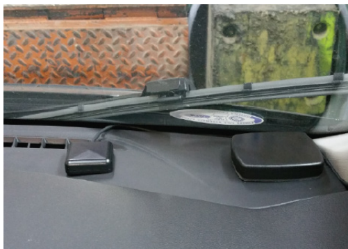
CRXS GPS and LTE antenna properly installed on the vehicle dash
