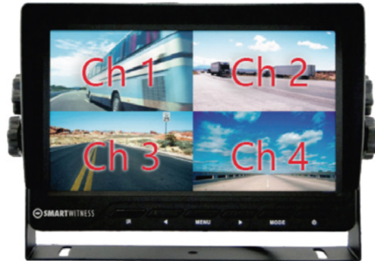
LCD camera channel display order (quad view)
