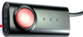
M1 button for G-sensor calibration
