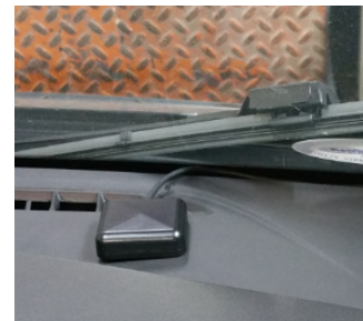
CP4S GPS antenna properly installed on the vehicle dash
