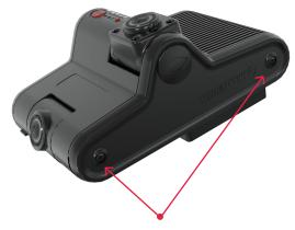
Unscrew the right-side bracket. Remove the KP2 from the bracket to adjust camera angle or insert/remove SIM/SD card.
