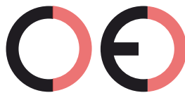
False CE Mark (too far)
